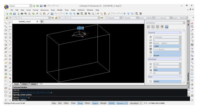
The Dynamic CCS can be turned on or off from a toggle in the bottom of the User Interface or by pressing F6. When enabled the CCS gets aligned to the surface automatically as you move over it.
