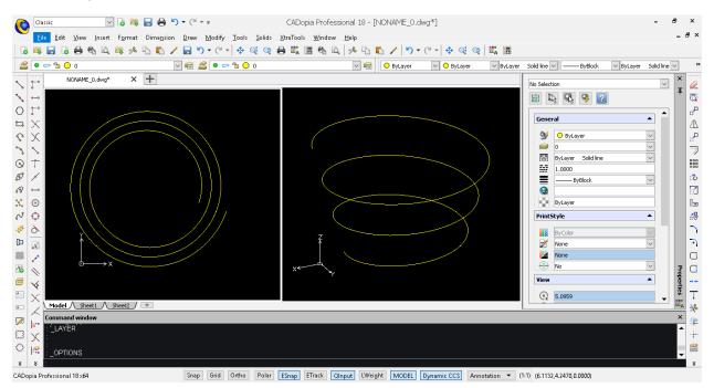
The HELIX is a new entity that can be used in 2D to create spirals or in 3D to create helices. You may further use an HELIX as an extrusion path and create complex shapes such as bolt threads, circular stairs or ramps.
